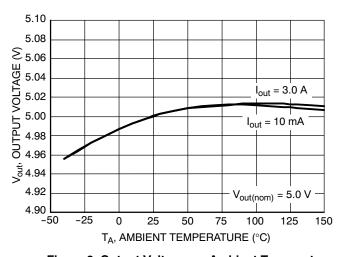
Figure 3. Output Voltage vs. Ambient Temperature
