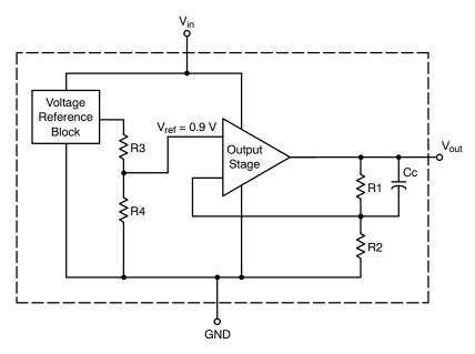
Figure 2. Block Diagram
