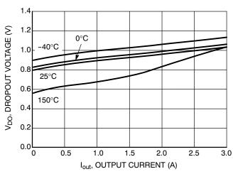
Figure 2. Dropout Voltage vs. Output Current
