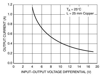
Figure 6. Output Current vs. Input-Output Voltage Differential
