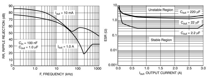
Figure 7. Ripple Rejection vs. Frequency
