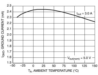
Figure 4. Ground Current vs. Ambient Temperature
