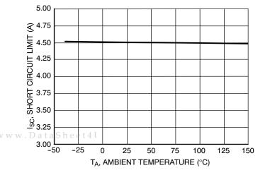
Figure 5. Short Circuit Current Limit vs. Ambient Temperature
