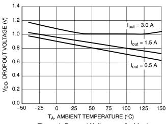
Figure 1. Dropout Voltage vs. Ambient Temperature
